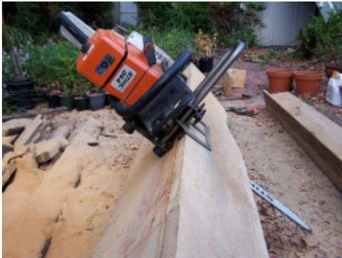
The timber guide can then be removed and successive boards cut off using the dimension plate. The plate can be easily adjusted out to about 20cm.
