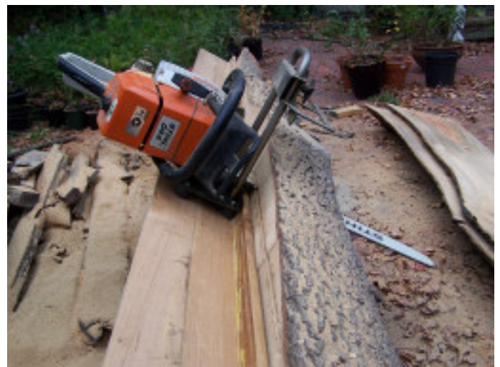
The second cut: the guide is put against the clean face to produce a right angle cut. Tilting the log makes holding the saw in place a little easier.
